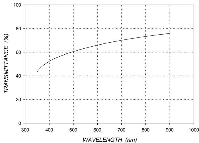
Fig. 2: Measured transmittance of (thickness of about of 400 nm) against wavelength. The reference wavelength is 632 nm (normal incidence).
